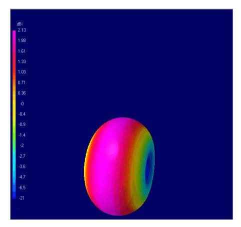
But that is only the case in 'free Space'. If you are working with NASA and plan to use that dipole out in the vacuum of space, you have the exact correct model in mind. If you intend to use your dipole a bit closer to the good old terra firma, your dipole won't radiate at all like that!
