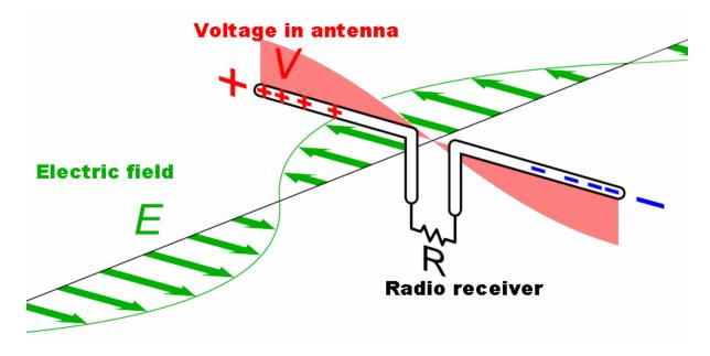
Most Hams are aware of the simple, 'back of the envelope calculation for the approximate length of a resonant center fed dipole:
