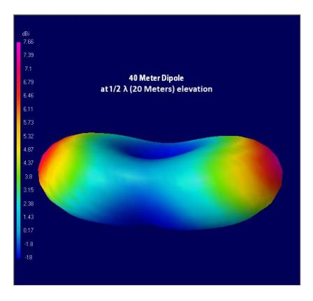
Notice how the high-energy lobes are pointed just a little bit up (keep in mind that the red-colored part has a lot more RF energy than the blue-colored portions)? Right at that lovely horizon so that the iono-sphere can let your signal reflect and refract that signal all over the world!
