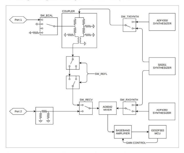
The S-A-A-2 is a single switched receiver VNA. While the diagram shows only two channels selectable by the receive mixer through SW\_RECV, a third channel, the reference channel, is provided by setting SW\_ECAL to the "open circuit" position. By controlling these two switches the receiver is able to observe reference, reflected, and thru signals.
