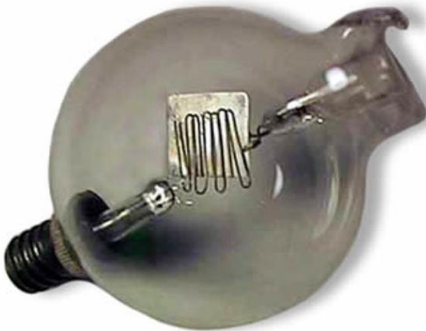
Lee DeForest's Audio Tube – The First Triode Vacuum Tube
