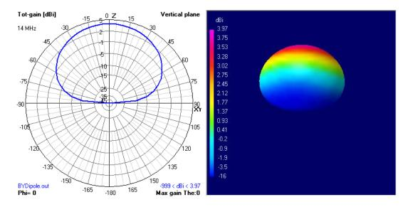
Now you can clearly see that most of your RF is shooting out of your dipole STRAIGHT UP! NVIS, pure and simple.
