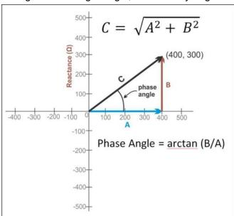
So, the impedance of your dream,  $Z = 50 + j\mathbf{0}$  can also be written as Z = 50 ohms with a 0-phase angle, or '50 ohms of purely resistive Impedance'.
