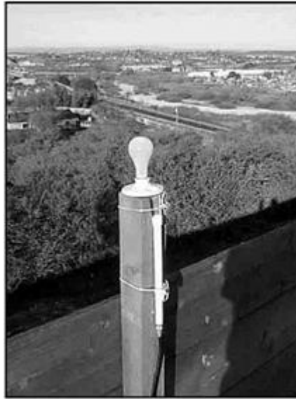
A single Illuminator. Notice the balun attached to the side of the post.
