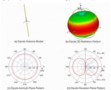
Most people call it *doughnut shaped*, I prefer *bagel shaped*. The maximum current is near the center feed and that's where most of the signal is radiating from (that's why an inverted "V" has better elevation than a simple "V" shaped dipole. The outer edges have the maximum voltage, so stay away from them when your transmitter is on. RF burns can be painful!
