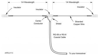
When you cut the wire lengths for the longest length you can mount, it is usually called a non-resonant *Doublet* or simply a *Doublet*. When it is measured and cut to be at a specific electrical resonance length for a favorite frequency, it is usually called a *Dipole*. How do you find "the right length"? Well, there's a story about that...
