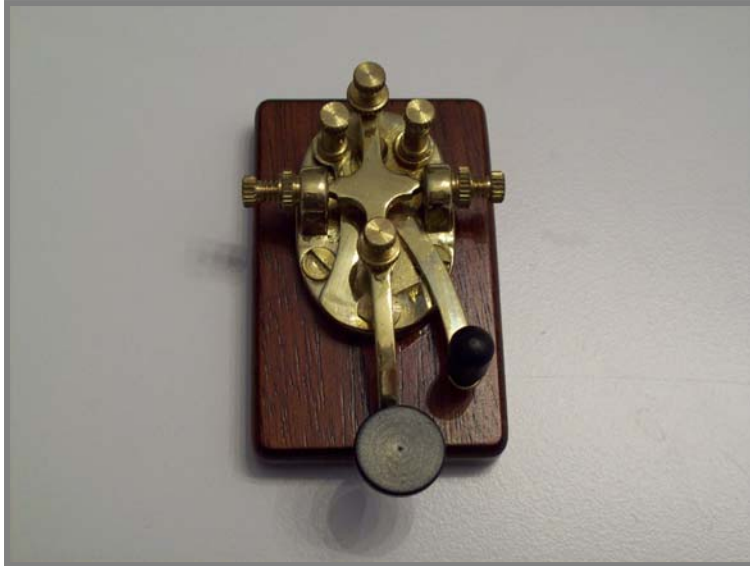
Photo 1 Note the circuit closing lever or "Bail Out Switch" on right side of this classic style pump/hand key. Does lack of said switch on modern keys indicate our stalled economy has been bailed out for the last time?
