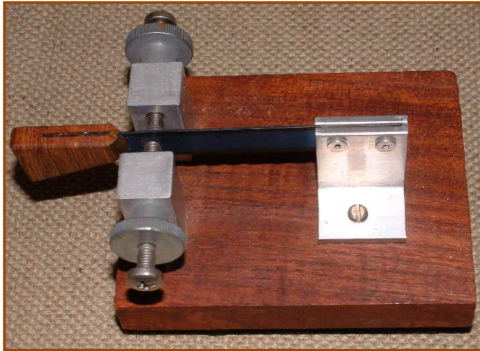
Photo 3 A number of amateurs use a hand-cut wood base and fingerpiece, metal angle brackets and pillars plus steel screws and a hacksaw blade to home-assemble their own Sideswipers—and they work good. Average length of hacksaw blade from bracket to fingerpiece is 3.25 inches for best “feel”.
