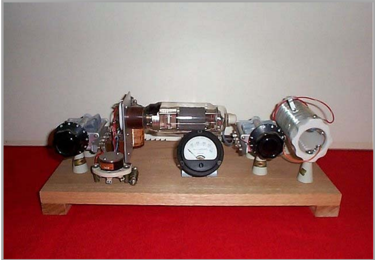
A big-time oscillator/transmitter from the 1930s. It used a type 804 tube. Photo courtesy of W6JRY.
